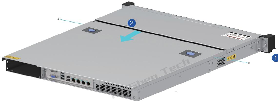
1. Loosen the screws at both ends of the upper cover as shown in the diagram, using your hands;
