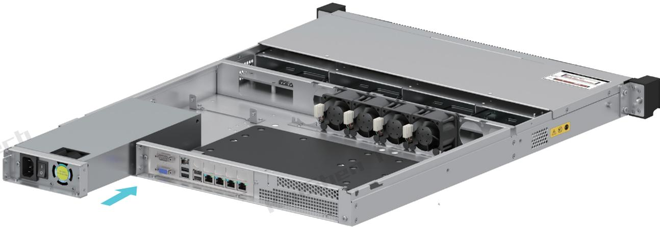
Install the power supply in the direction of the arrow
